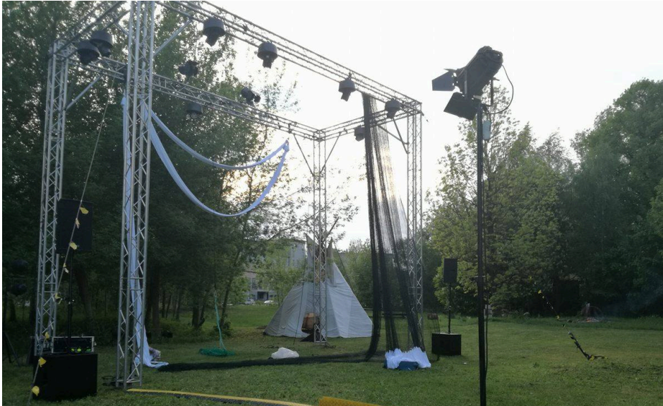
example of truss rigging
